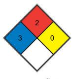
Short exposure could cause serious temporary or moderate residual injury (e.g. <u>liquid hydrogen, sulfuric acid</u>, <u>calcium</u>
