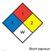
Short exposure could cause serious temporary or moderate residual injury (e.g. <u>liquid hydrogen, sulfuric acid, calcium hypochlorite</u>, hexafluorosilicic acid)
