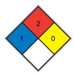
HEALTH 1 Exposure would cause irritation with only minor residual injury (e.g. <u>acetone</u>, sodium bromate, potassium chloride)
